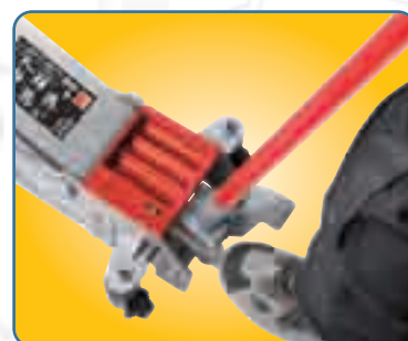
PEDAL TO DISCONNECT THE SAFETY BLOCK
